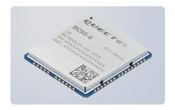
BC95-G is a high-performance NB-IoT module which supports multiple frequency bands of B1/B3/B8/B5/B20/B28\* with extremely low power consumption. The ultra-compact 23.6mm × 19.9mm × 2.2mm profile makes it a perfect choice for size sensitive applications. Designed to be compatible with Quectel GSM/GPRS M95 module in the compact and unified form factor, it provides a flexible and scalable platform for migrating from GSM/GPRS to NB-IoT networks.
