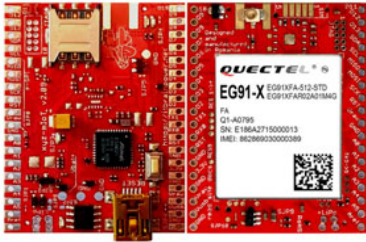
xyz-mIoT equipped w. EG91E modem LTE CAT1 + 3G + 2G European (EMEA)
